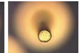
Circle probe appears on the abnormal pin location without measurement failure
