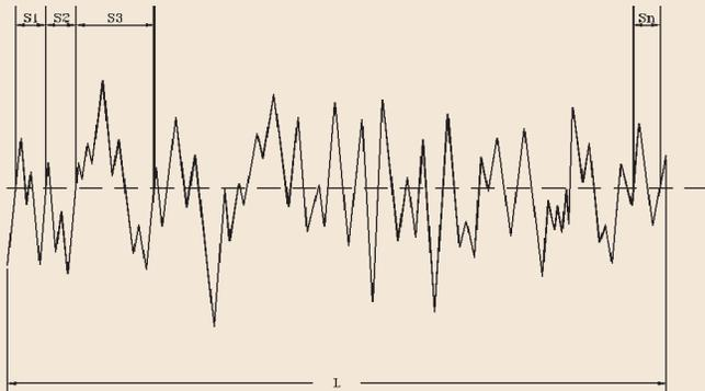
**Mean Spacing of Profile Irregularities,  $S_m$** , is the mean value of the spacing between profile irregularities within the evaluation length.
