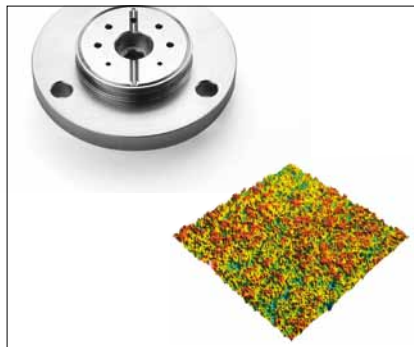
Titanium Texture analysis of a chemically polished surface (DHM S2)
