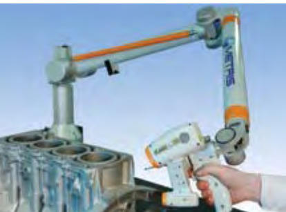
MMD scanner is available in 50/100/200 stripe width and scans at maximum rate of 80,000 points/sec
