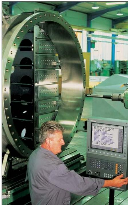
Frequently recurring machining sequences are saved as **fixed cycles**.
